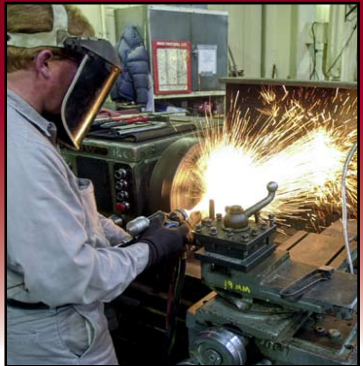
Flame spraying bearing fit with wire feed cool spray system.
