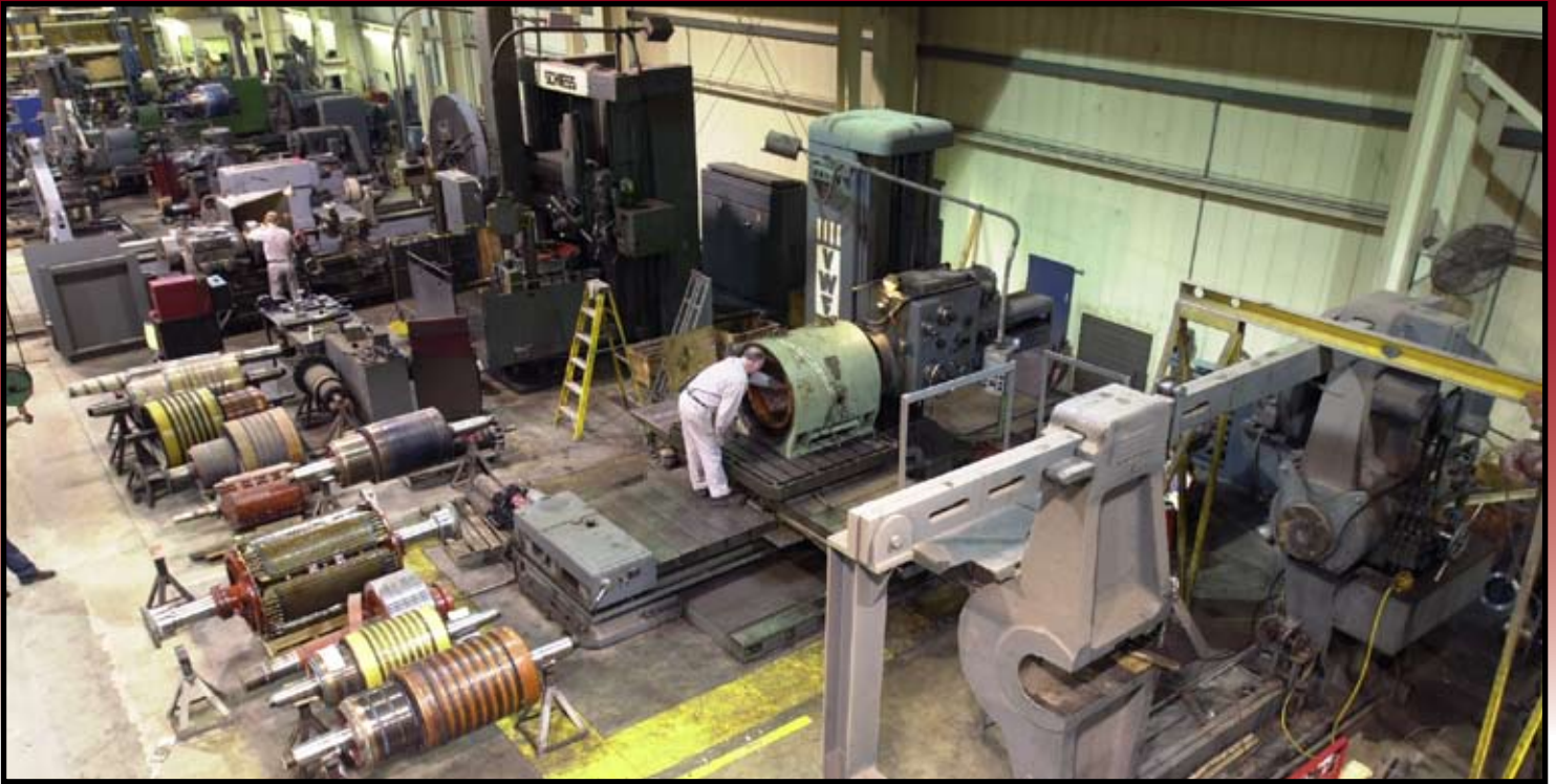
Horizontal millwork includes repairing stator registers and facing stators.
