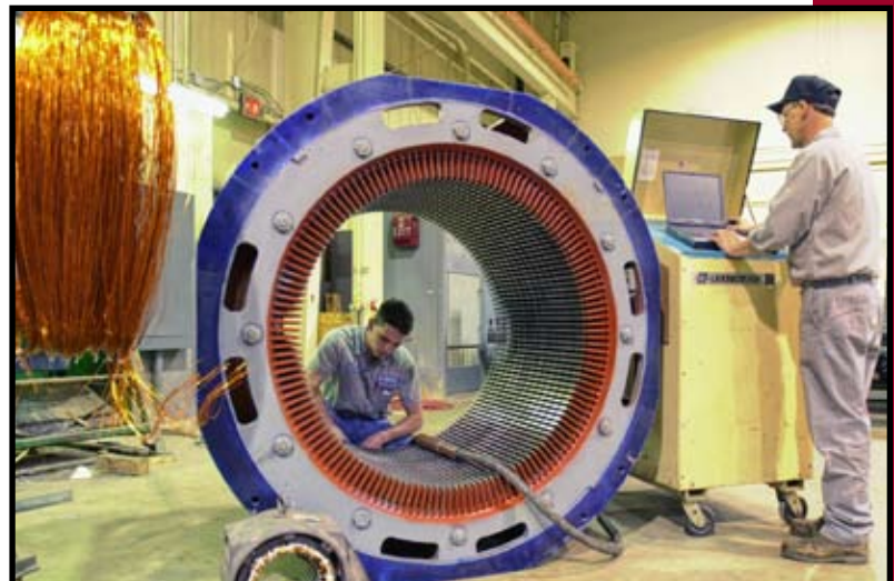
Performing core loss test on a large AC stator.
