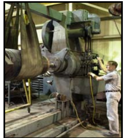
Our 1,000-ton horizontal press pushes a shaft out of a 622 armature.
