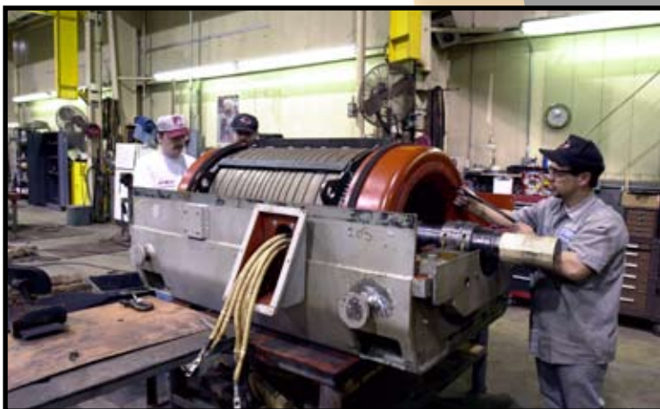
The air gap on a 1,250-hp AC motor is adjusted.
