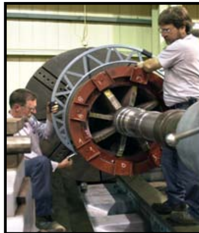
Machinists mic the outside diameter of a 6,000-hp rotor.
