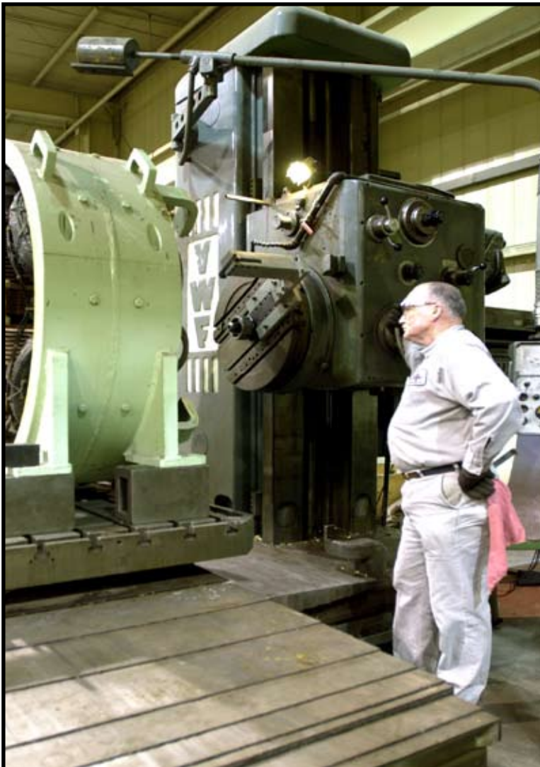
Brush ring mounts being machined on a large generator frame.
