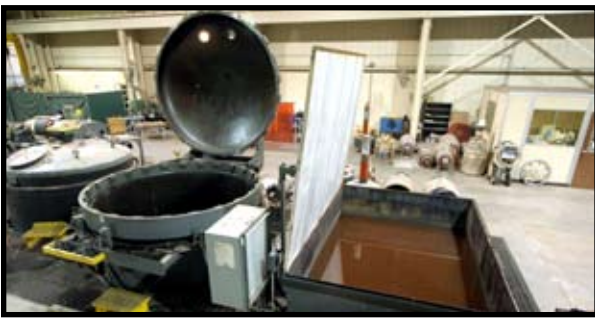
8' epoxy VPI system, 5' polyester VPI system, and 12' x 8' dip tank with epoxy overdip resin.
