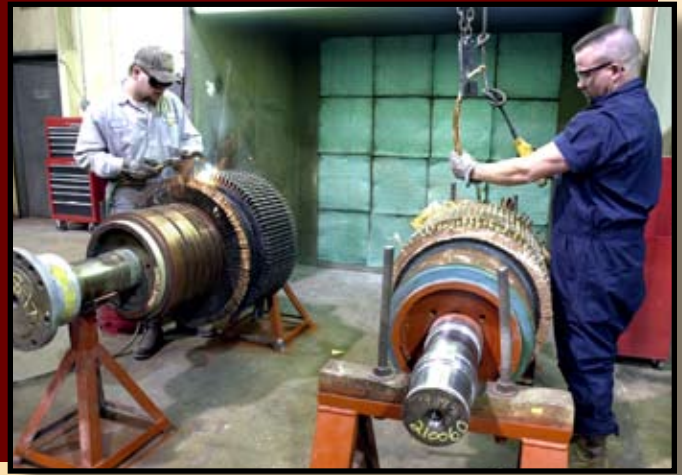
Armatures are stripped with care to ensure the highest quality.
