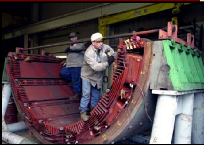
Flanders removes and rebuilds motor coils with very little downtime for the consumer.
