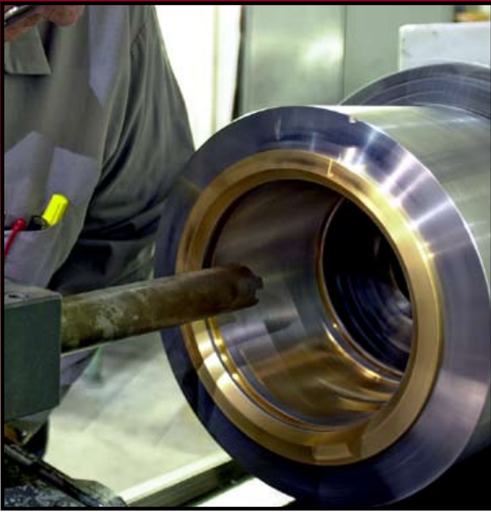
The Flanders machine shop includes a complete Babbit bearing facility.
