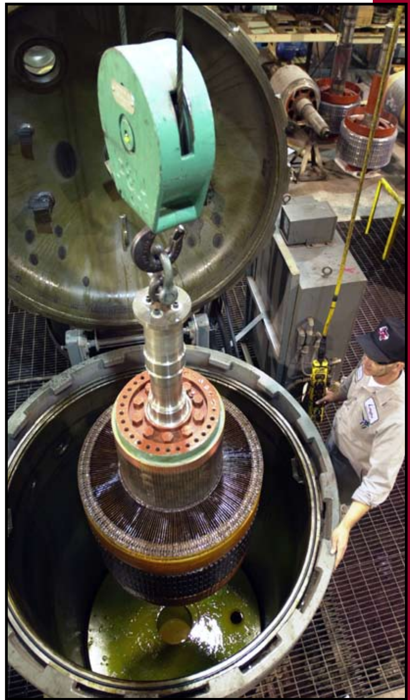
Armature being prepared for vacuum-pressure-impregnation.
