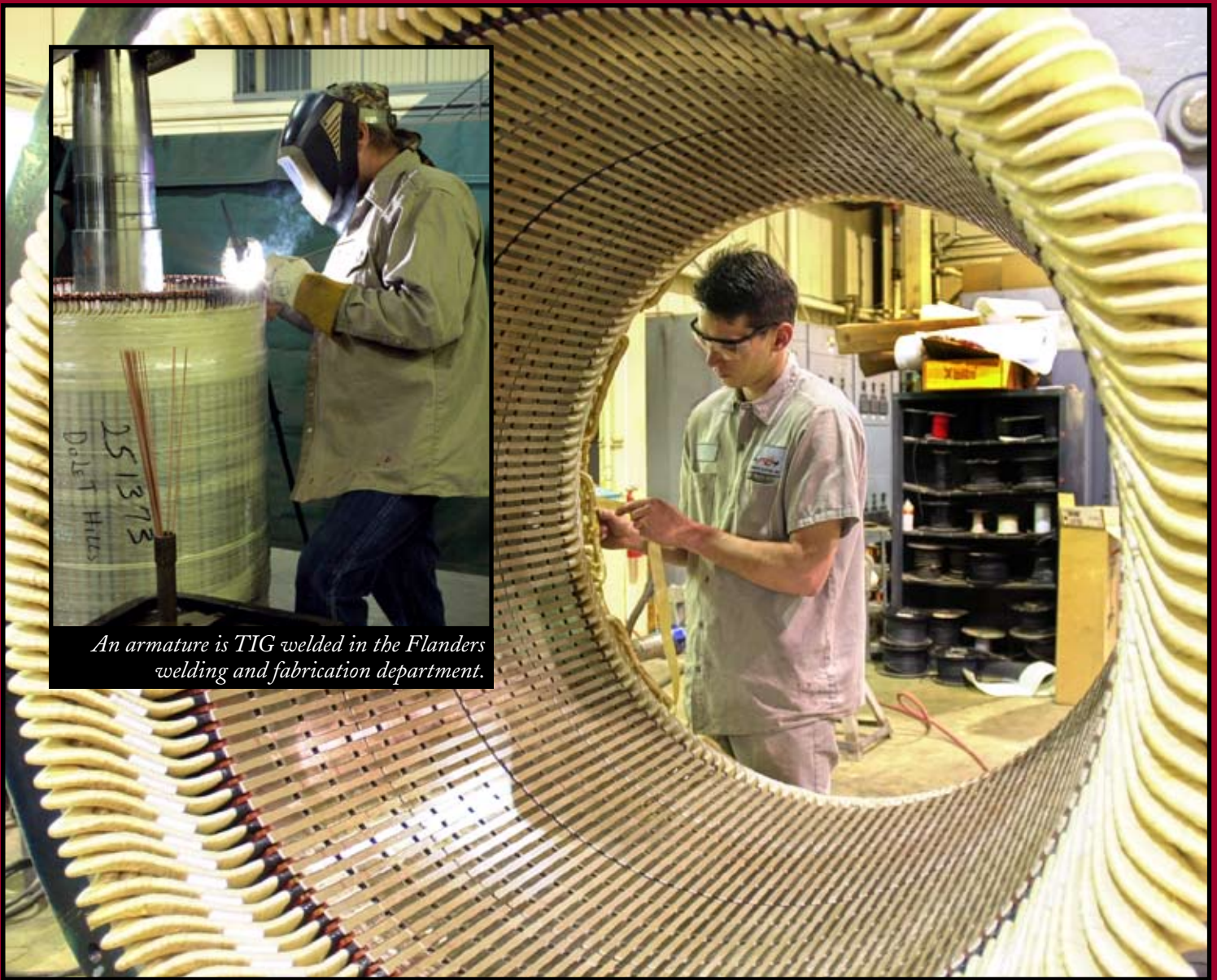
A technician tapes connections on a 3,500-hp synchronous stator that runs at 6,600 volts.
